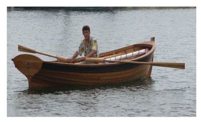
Classic navy four oars skiff. The hull is made of solid oak and pine (Oak framing and fir or pine planking). Six Ash oars. Sprit foresail. Spars made of pine. Stainless steel hardware. Oak rudder.
